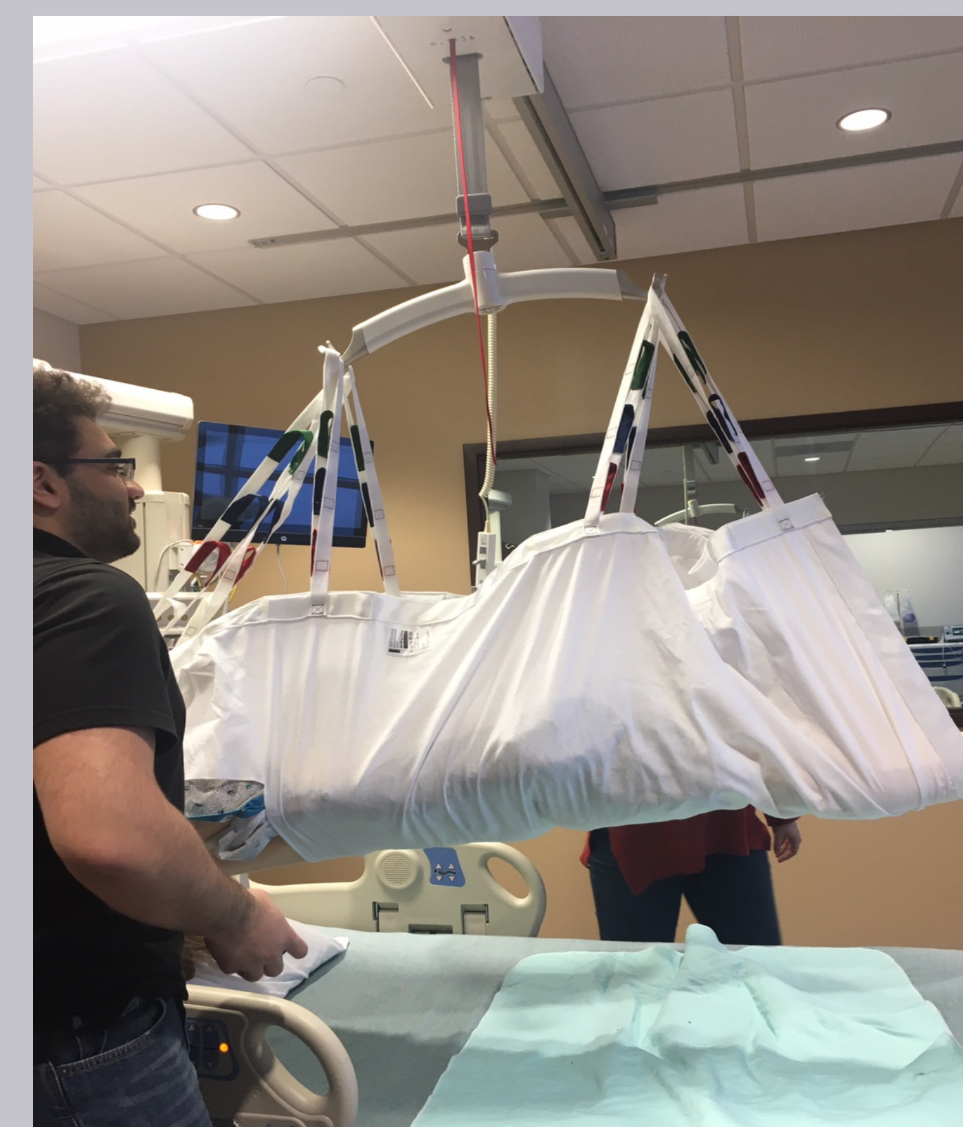
Figure 3. This is the current sling being used with the ceiling lift at the Mirro Center at Parkview Hospital.
