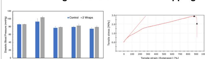
The TPU filament bandage demonstrates an ability to withstand 190.81 N before it slips during experimentation. The diastolic pressure data illustrates an increase in application pressure by measuring the differences in blood pressure between the control (no wrapping) and two wraps of the final bandage design. The difference in diastolic pressures is not statistically significant. The bandage is not restricting blood flow to the distal portion of the arm.
