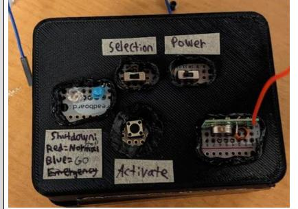
Using a single-core wire, the transmitter has a monopole quarter wave antenna with a range of 54 feet.
