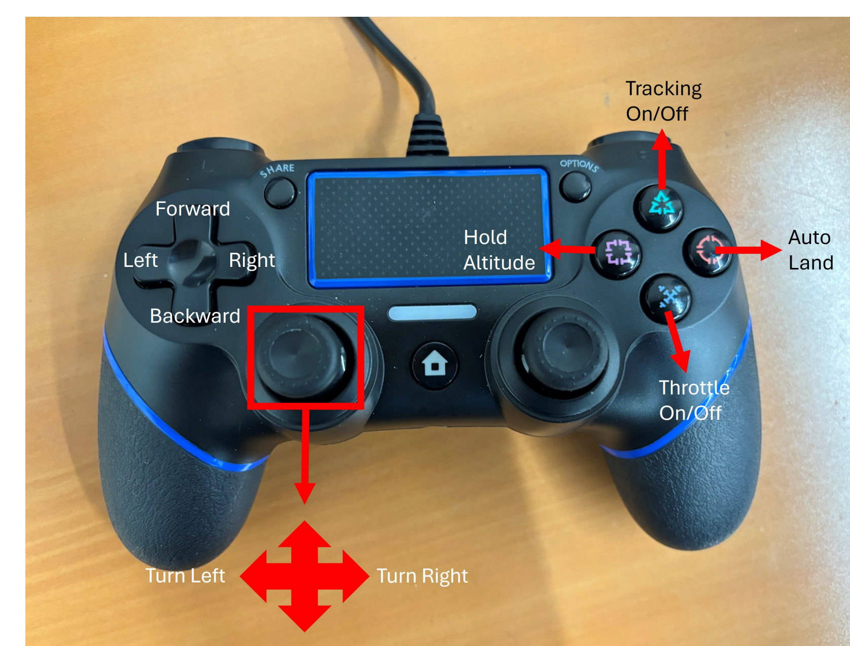
Figure 3: Controller's button and joystick functions
