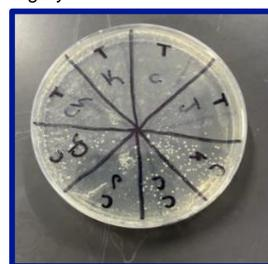
12 trials of sterilization were performed. For each trial, the device was thoroughly scrubbed with microbial contaminants and swabbed to collect control samples on an agar petri dish. After autoclave each autoclave cycle, the device was swabbed again to observe if bacteria would grow in the test area of the petri dish.
