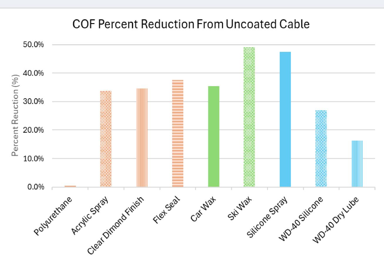
Based off COF reduction, the best coating we tested was Ski Wax and the Silicone Spray.
