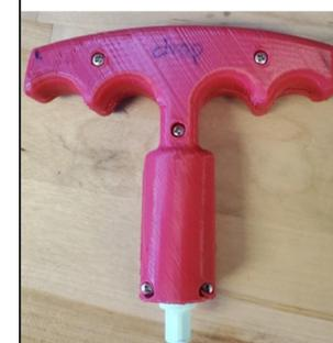
In conclusion, the most important problems this torque wrench could rectify are issues that current industry torque wrenches cause. Torque wrenches currently on the market rarely ever hit their manufacturing set torque limit even within a plus or minus 10% range. The main issues a disposable torque wrench will solve are lowering cost, increasing the accuracy of pre-set torque values and ease manufacturing processes for PMI while also improving
