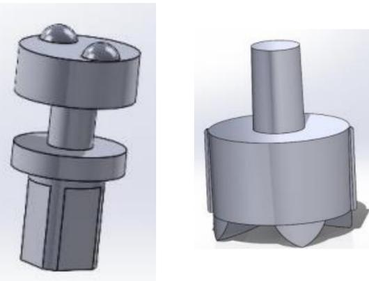
The final portion of the design includes a rough draft of the injection mold that will need to be created before production can start. The image below shows a rough draft of one half of the injection mold.
