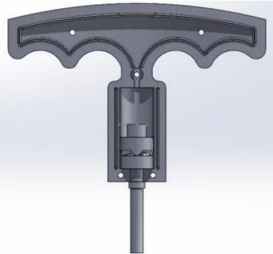
The two internal pieces were designed to interface with one another and at their peaks, the proper torque value will be outputted. The spring rests on top of the resistance plate and is further compressed when a torsional force is applied to the handle. Redesigns of the internal components included reducing diameters for better clearance, increasing thickness to increase compression, and changing the shaft end to accommodate for the testing methods required.
