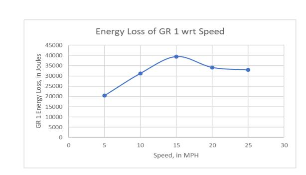
These plots depict the energy losses from the EV go-kart. As the plots illustrate, the energy loss from the kart is a function of the speed where, in general, the loss increases as the speed of the kart increases. Additional losses from the motor are included below: 5mph: 43507.67 J 10mph: 80249.69 J
