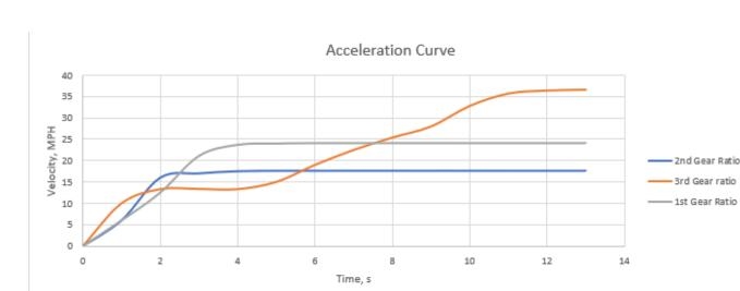
Based on this plot the most desirable gear ratio for the team to use would be the first gear ratio that was tested, 2.46. This gives the best balance of top speed and acceleration.
