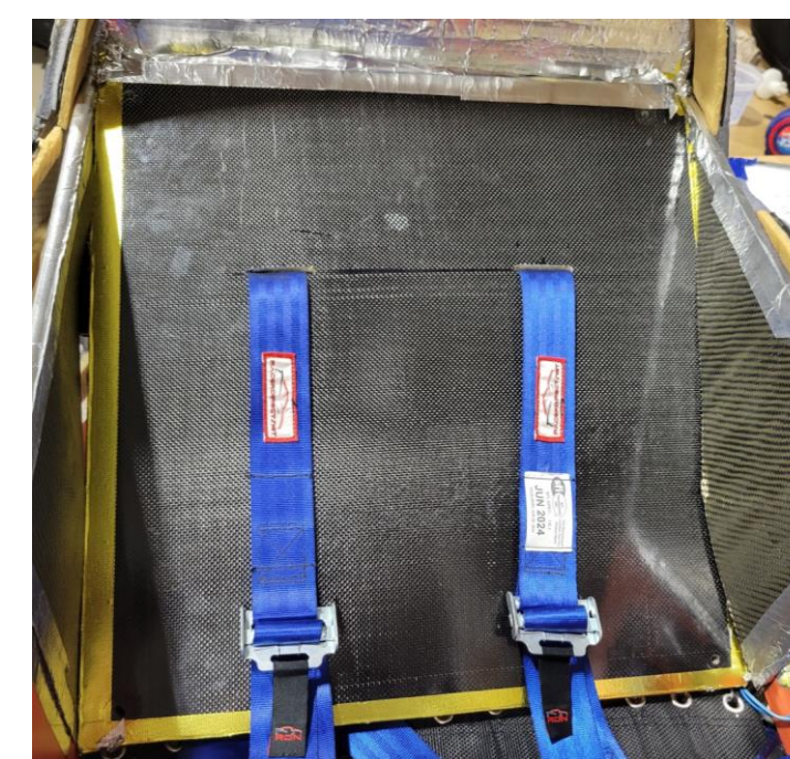
Finished and Installed Firewall
