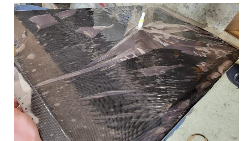
Vacuum Bagged Firewall
